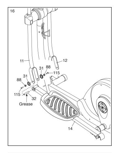
17. Lift the latch on the underside of the Left Pedal Arm (14), and set the Left Pedal Arm on the left Crank Bushing Sleeve (43).
