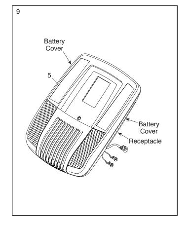
10. While a second person holds the Console (5) near the Upright (3), connect the wires on the Console to the Upper Wire Harness (48) and to the Pulse Wires (118).
