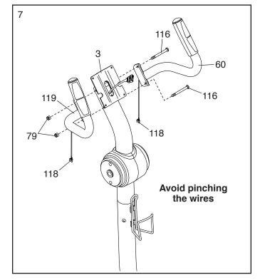
8. Insert the Pulse Wires (118) upward through the Upright (3) as shown.
